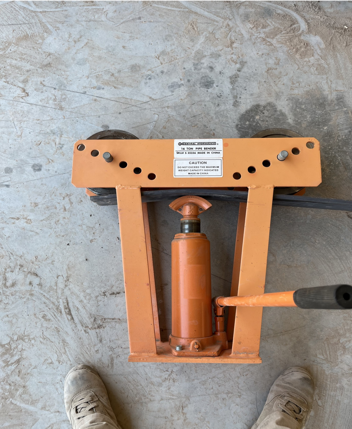
Figure 18. Demonstration of ability of the hydraulic tube bender to bend the 4" tall x 1/2" thick rail material.
