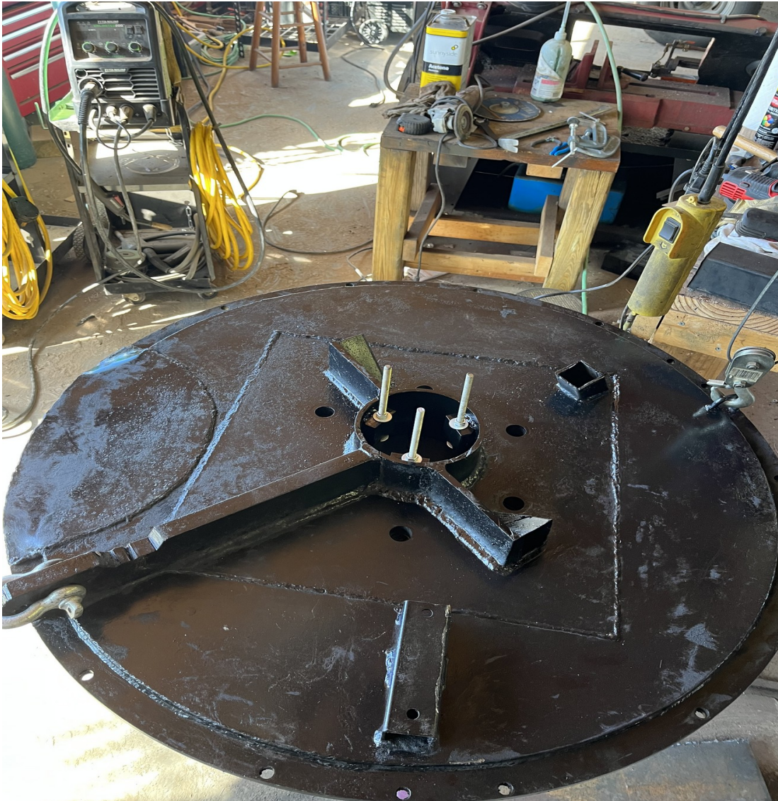
Figure 5. Three AZ encoder mounting posts have been installed on the top plate, ready to mount the encoder itself.
