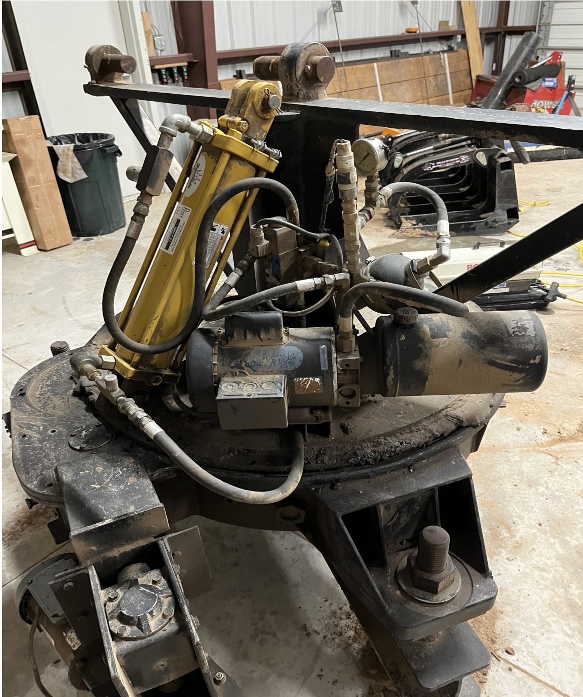
Figure 2. Original configuration of the AZ/EL mount previously used by the author.
