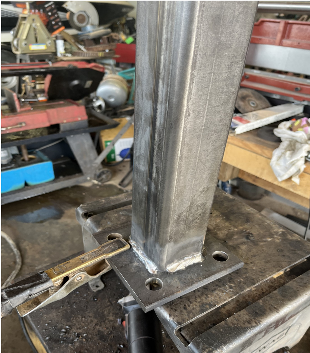
Figure 26. Showing how a flange plate is welded onto a rail support post.
