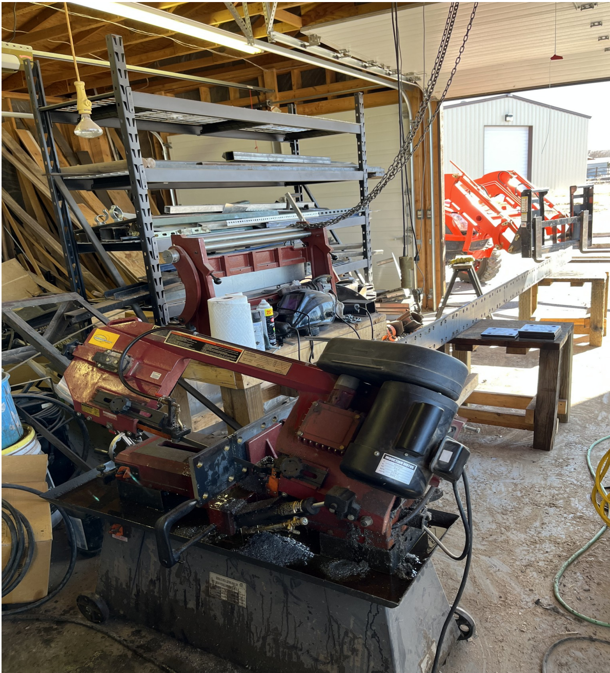
Figure 22. A flange plate is being cut from the 20' long steel bar. The saw blade is half through the plate as shown.
