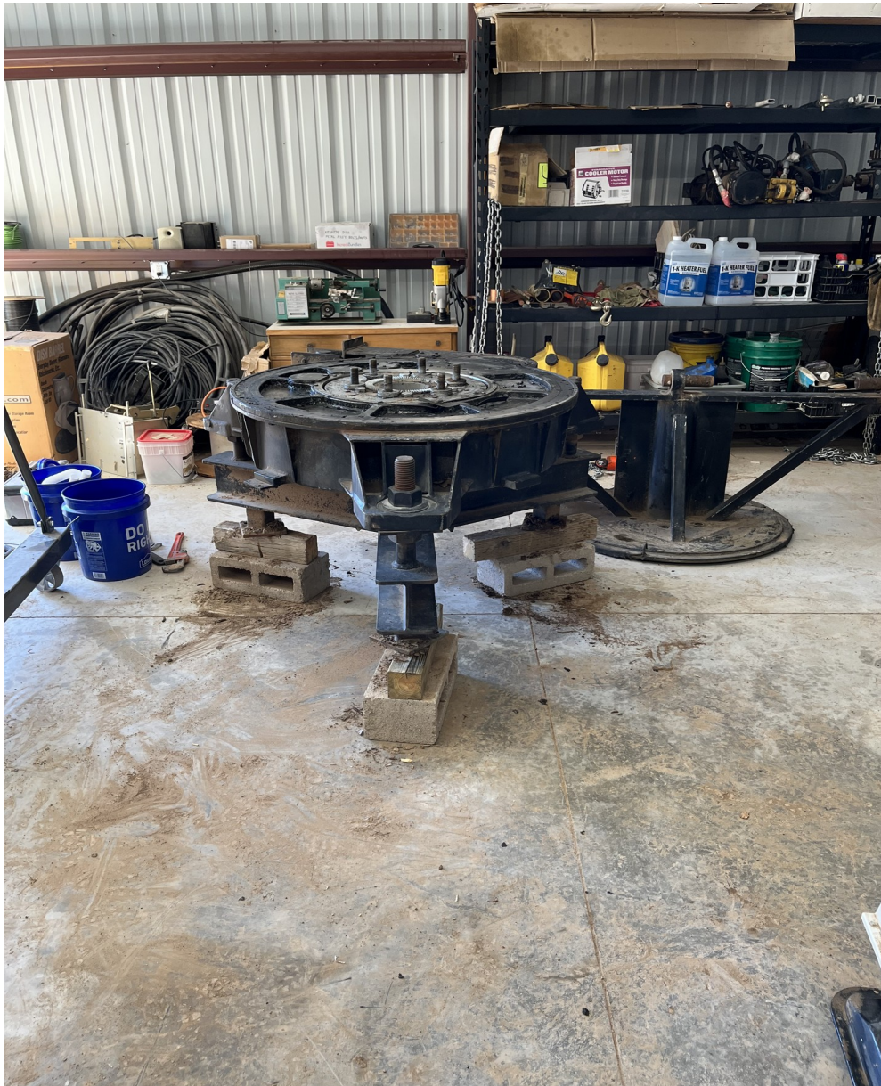
Figure 3. Original AZ mount shown with the top section cleared of hydraulic components and unbolted from the lower section.
