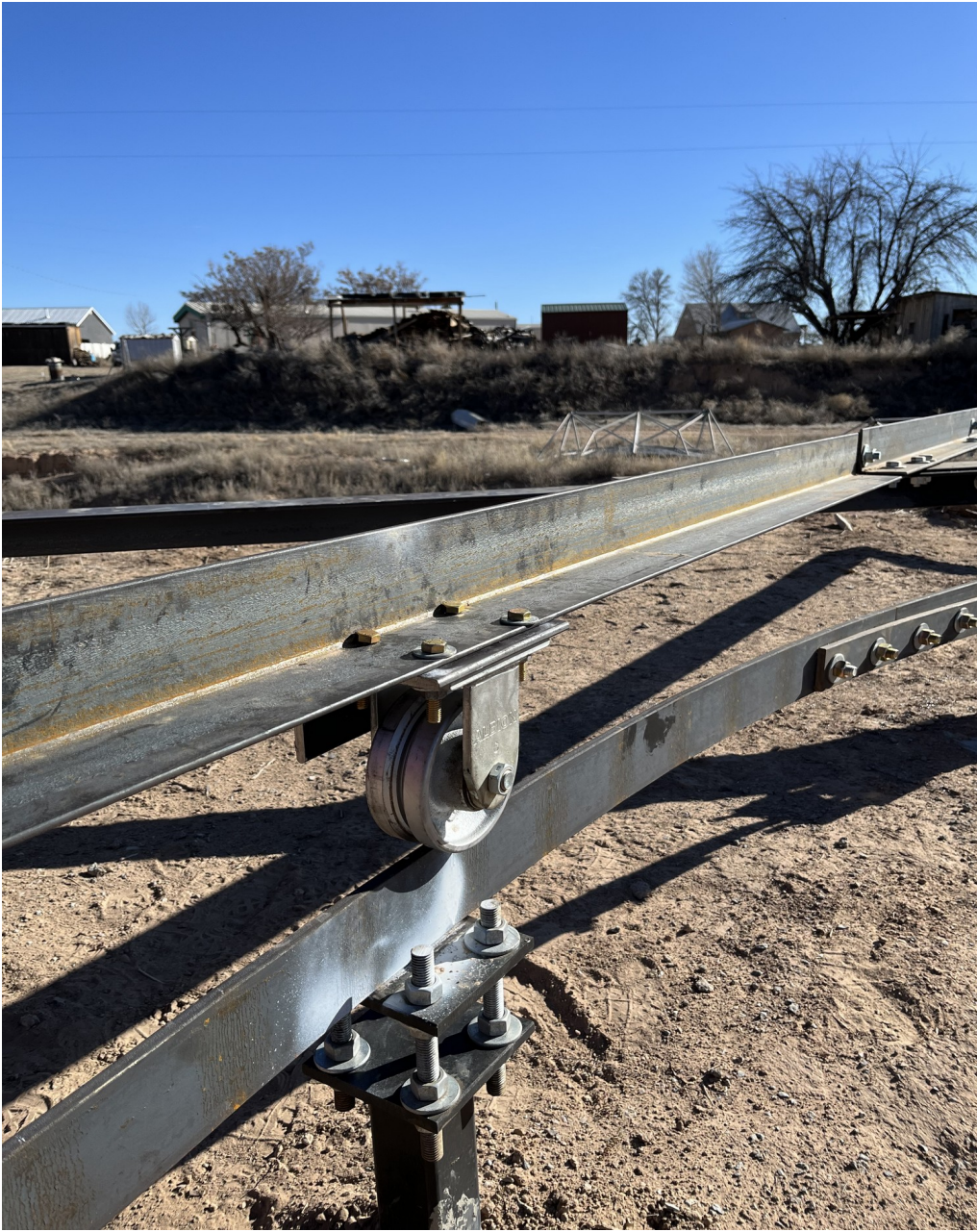
Figure 24. A wheel spacer is shown installed between the wheel assembly and the full square base structure.
