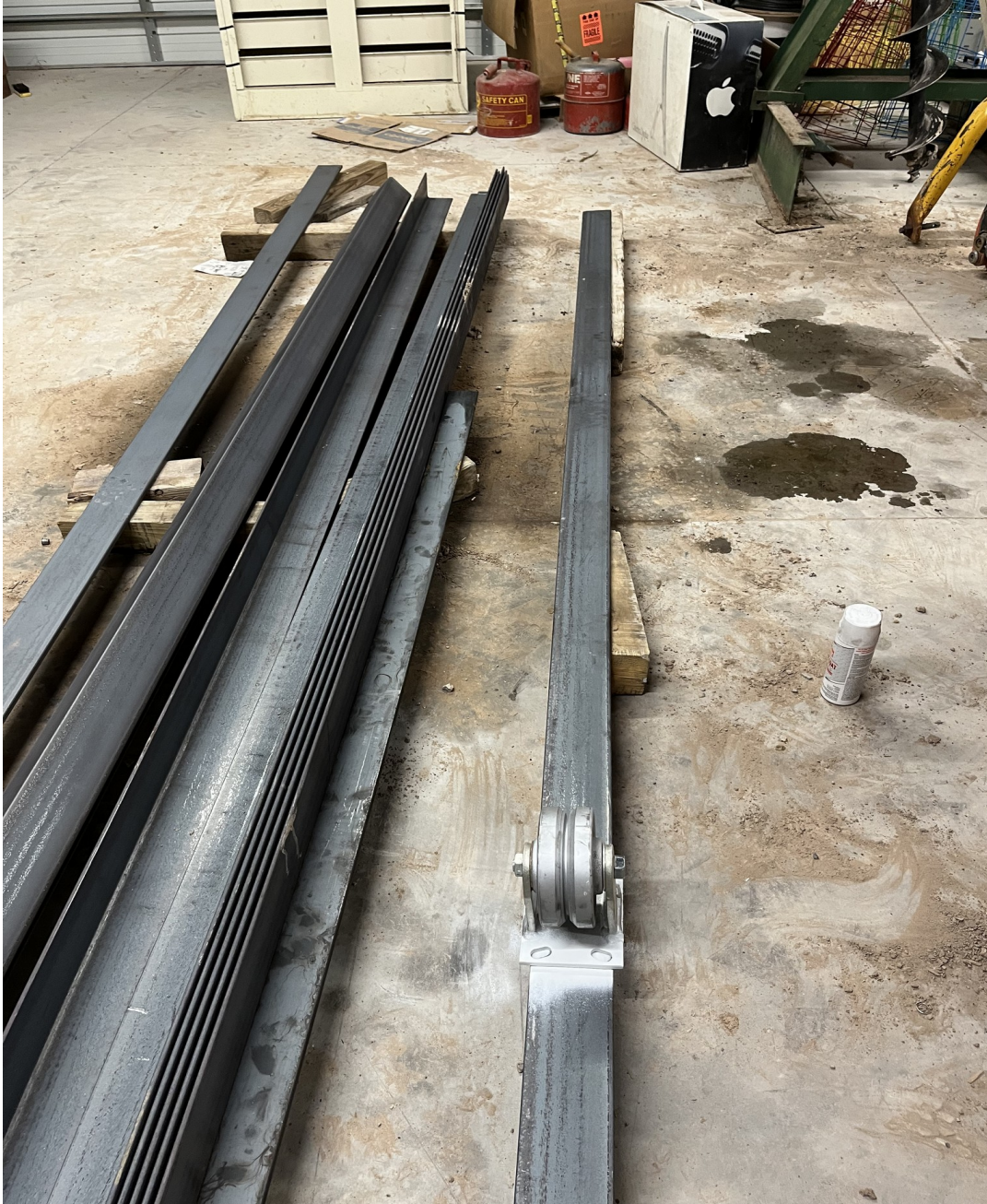
Figure 3. Spray painting the base of the wheel assembly to mark bolt hole positions.
