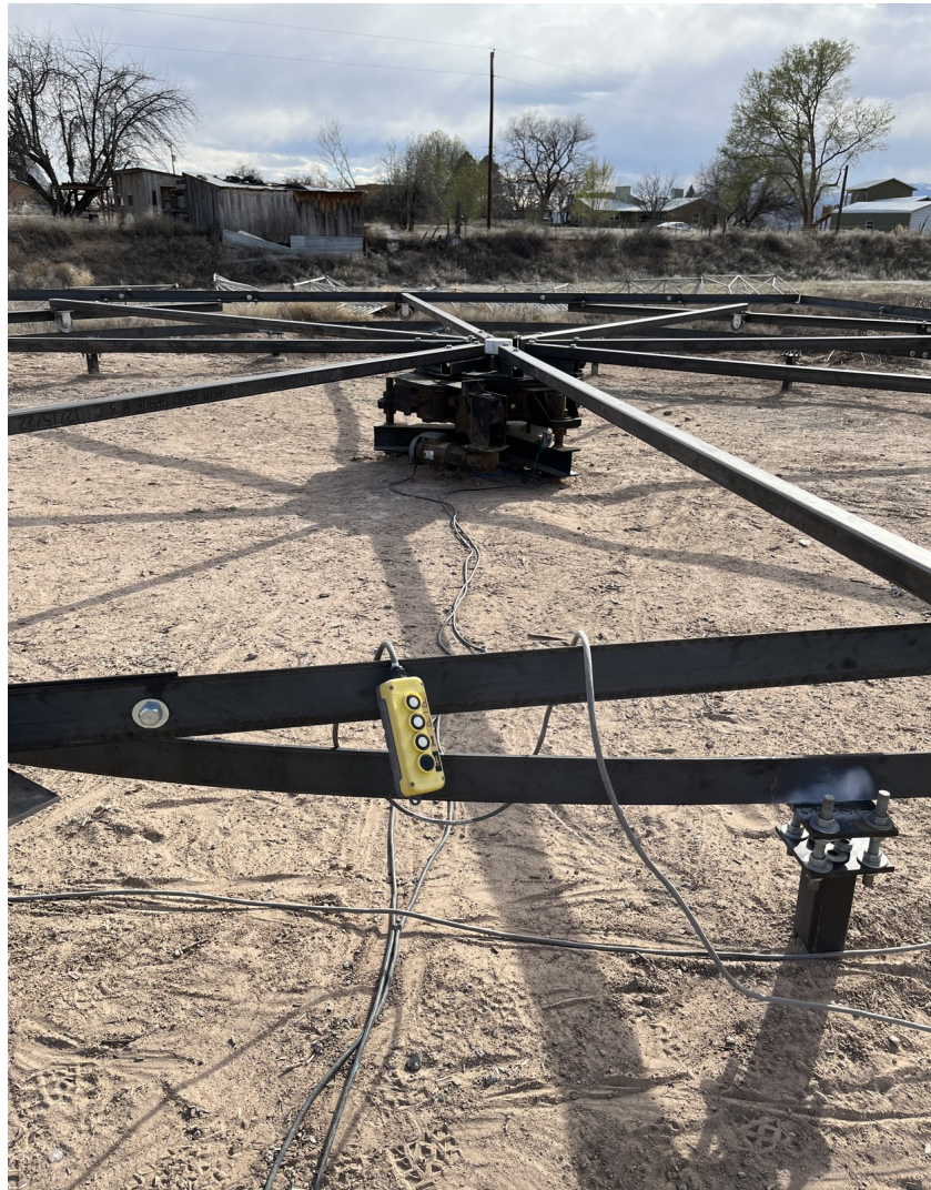
Figure 38. A hand-held remote control for the AZ mount drive has been installed to allow control of rotation locally while at the mount (13APR2023).
