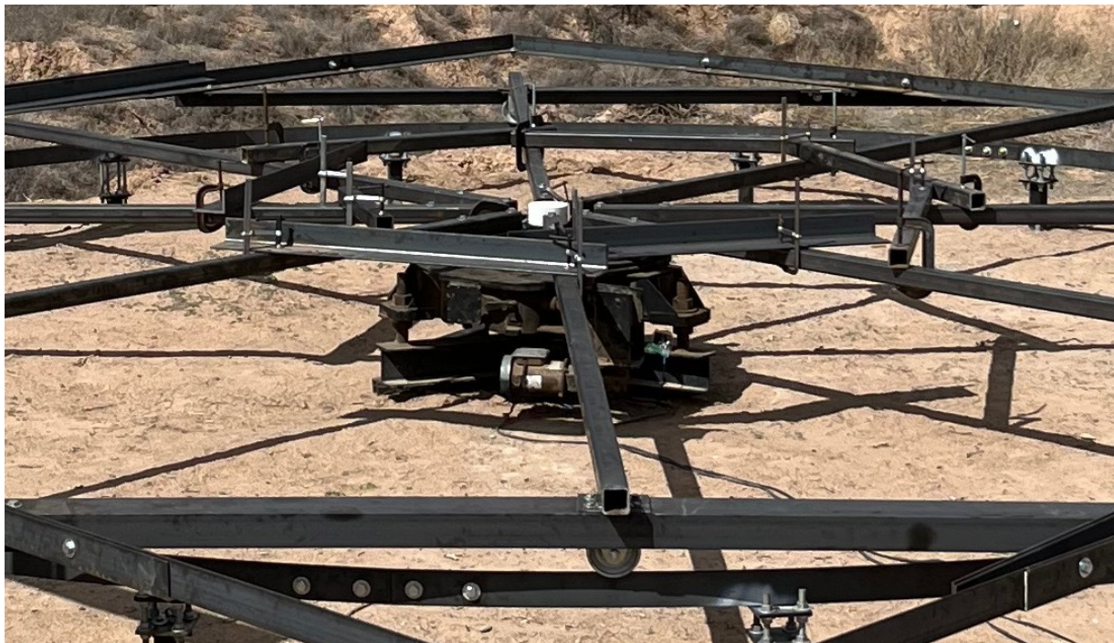
Figure 39. A set of various steel members were temporarily clamped onto the spokes, as shown, to check whether such members could stabilize the hesitation behavior observed without them.
