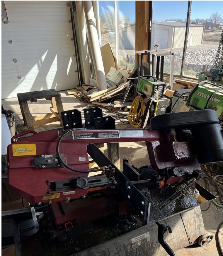
Figure 23. Using a metal saw to cut the four wheel spacers from angle steel.
