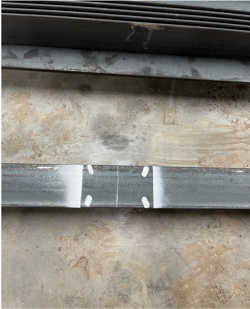
Figure 4. Center side piece with bolt hole positions marked.
