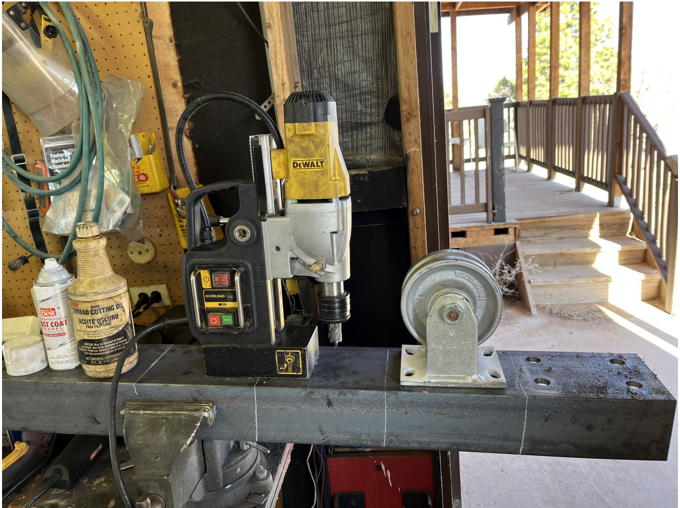
Figure 22. Setup to bore holes for the four wheel spacers.
