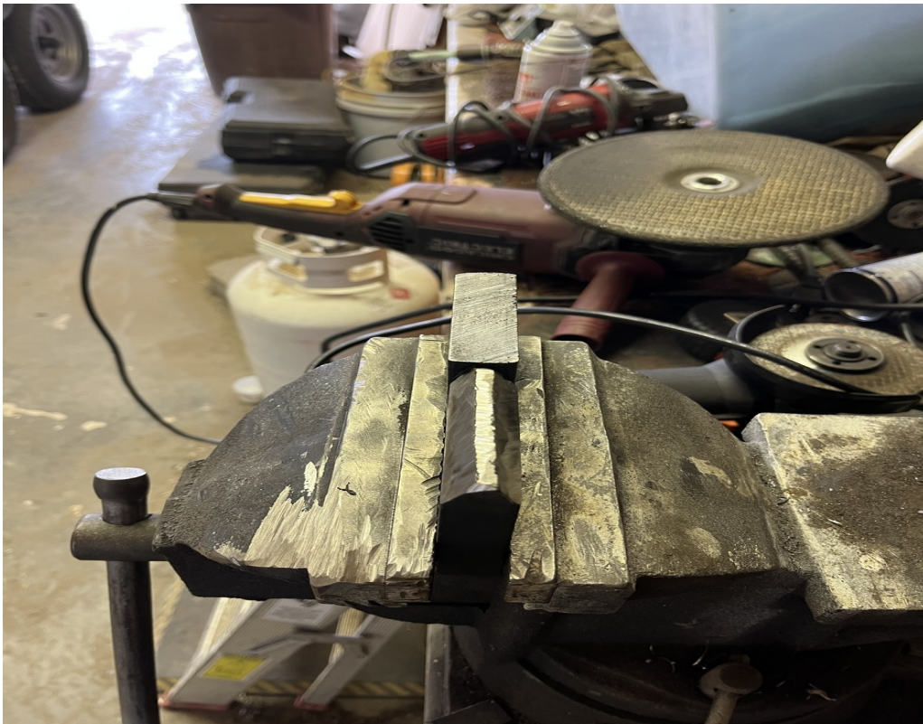
Figure 11. The two tabs are shown clamped in a vise with the joining ends protruding. One has been ground in preparation for a high-strength weld and the other is not yet ground.
