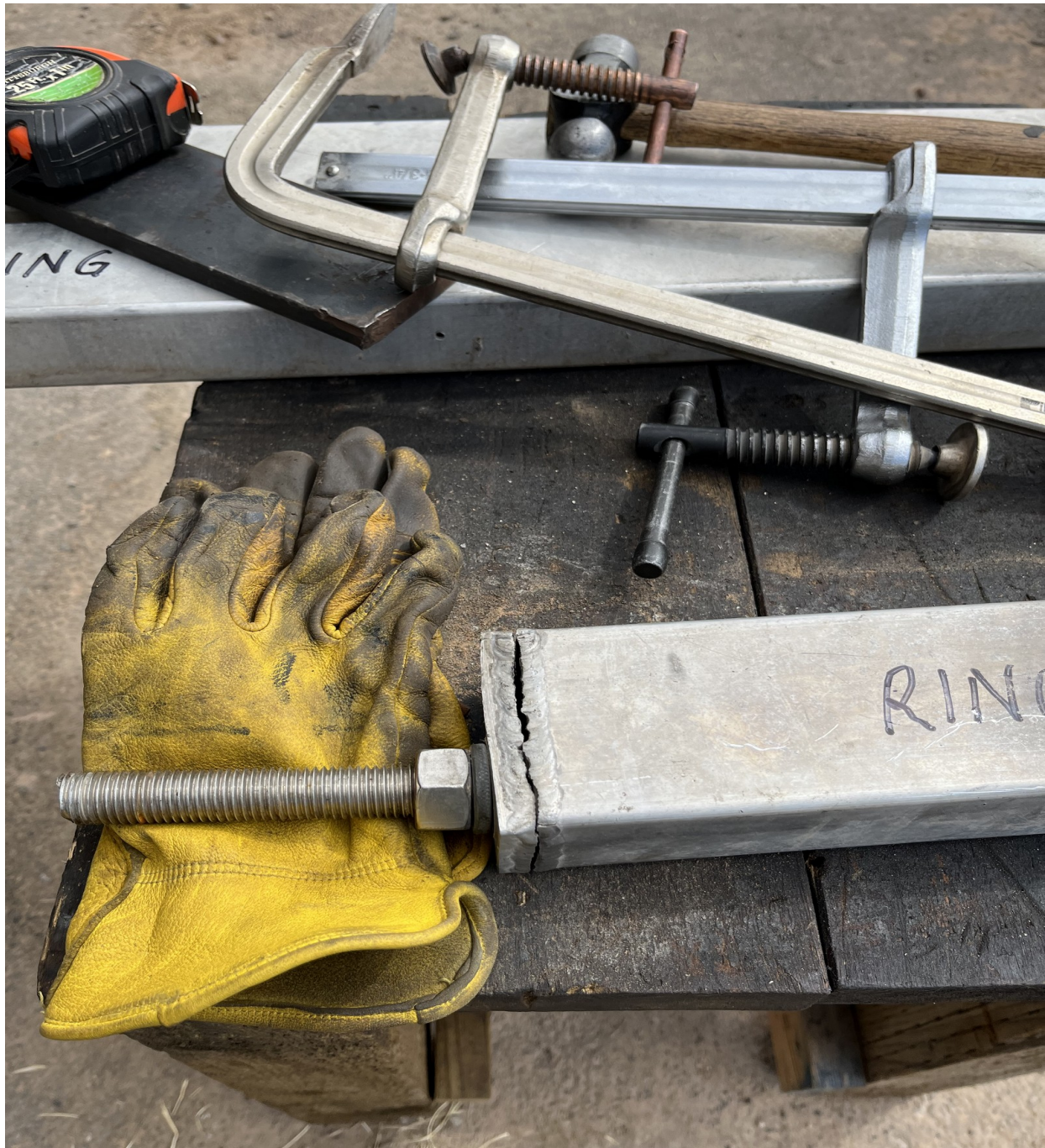
Figure 12. Broken end piece in position for welding (26JUL2023).
