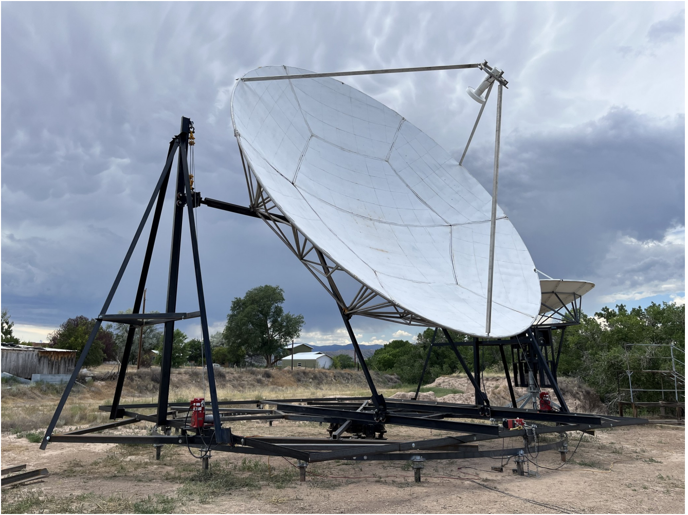
Figure 20. Dish is pointed skyward after installation of the feed horn (28JUL2023).
