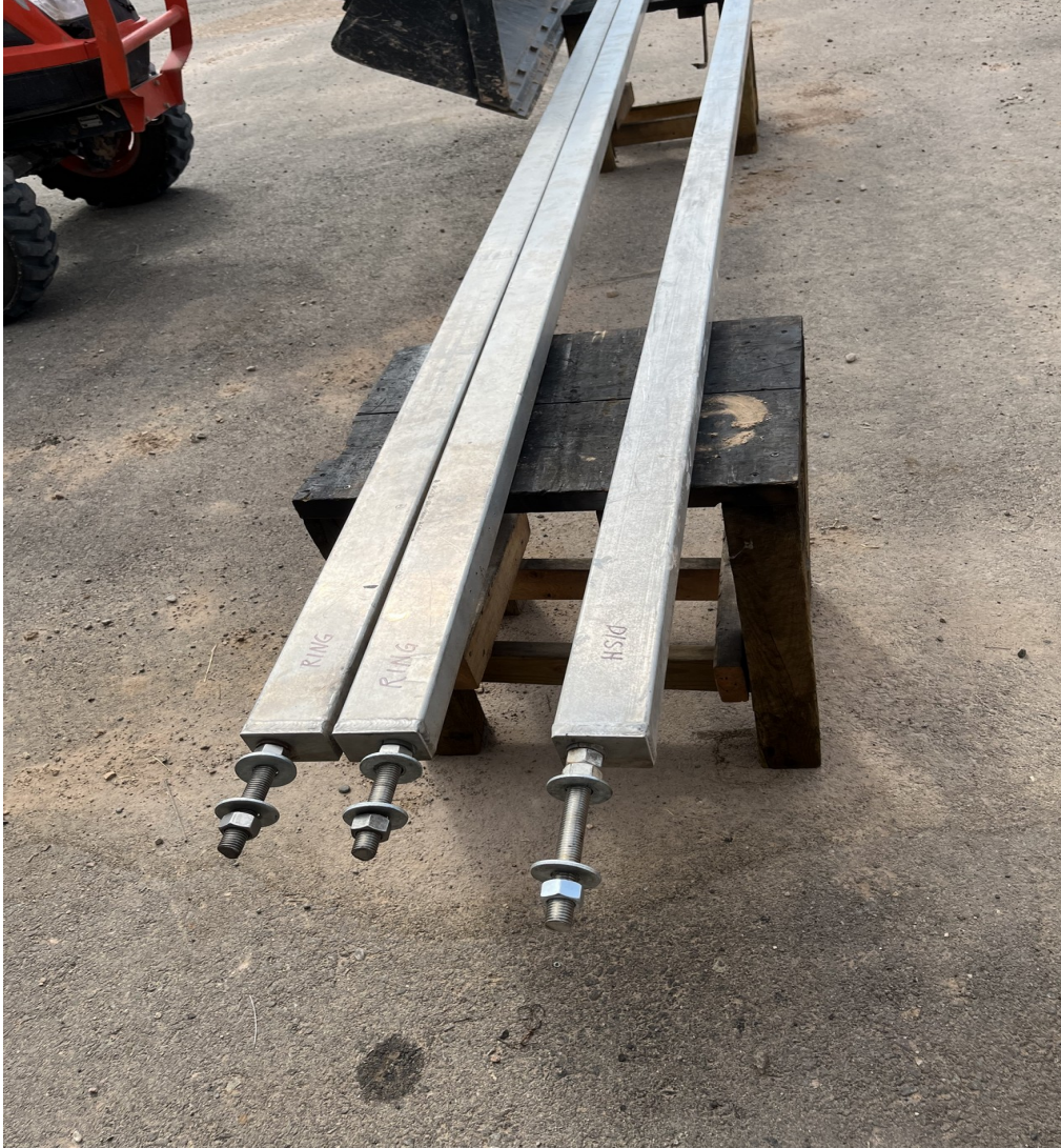
Figure 11. the previously bent threaded rods have been straightened without damaging the aluminum beams (26JUL2023).
