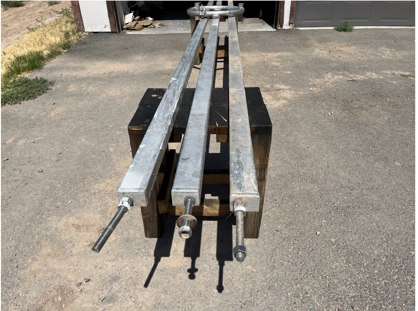
Figure 9. Dish rim ends of the feed horn support beams (25JUL2023).
