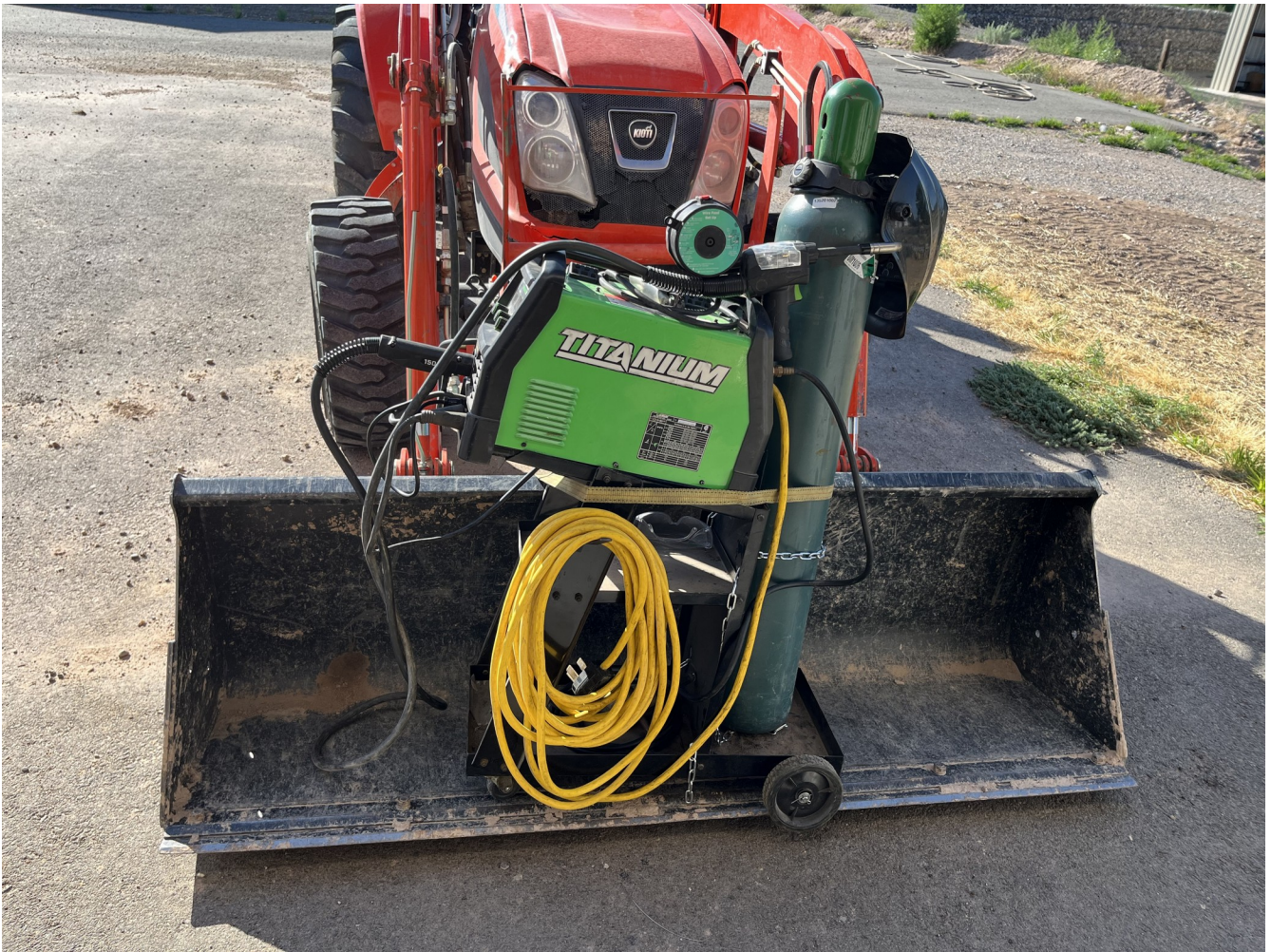
Figure 17. The MIG welder has been fitted with a spool gun and Argon gas bottle to weld aluminum (28JUL2023).
