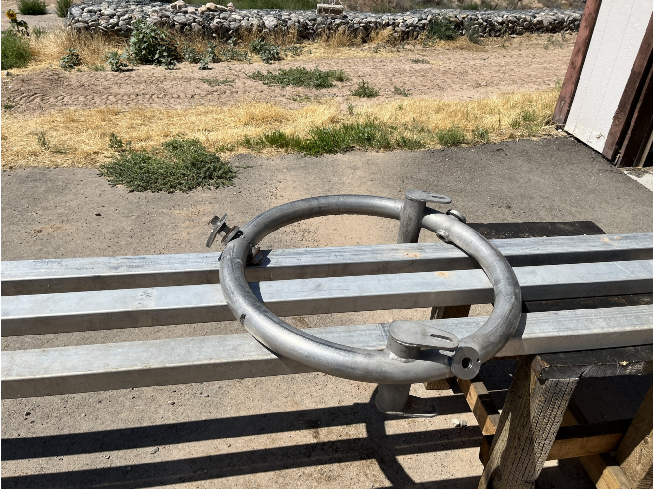
Figure 10. Feed horn mounting ring component of the feed horn support assembly (25JUL2023).
