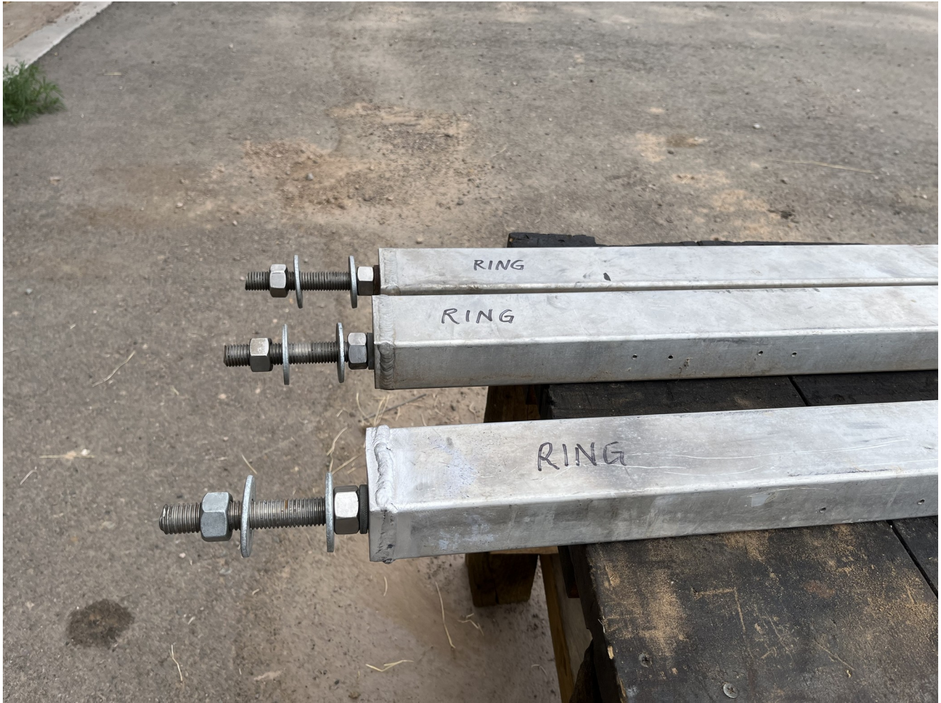
Figure 13. Repaired end piece after welding (26JUL2023).
