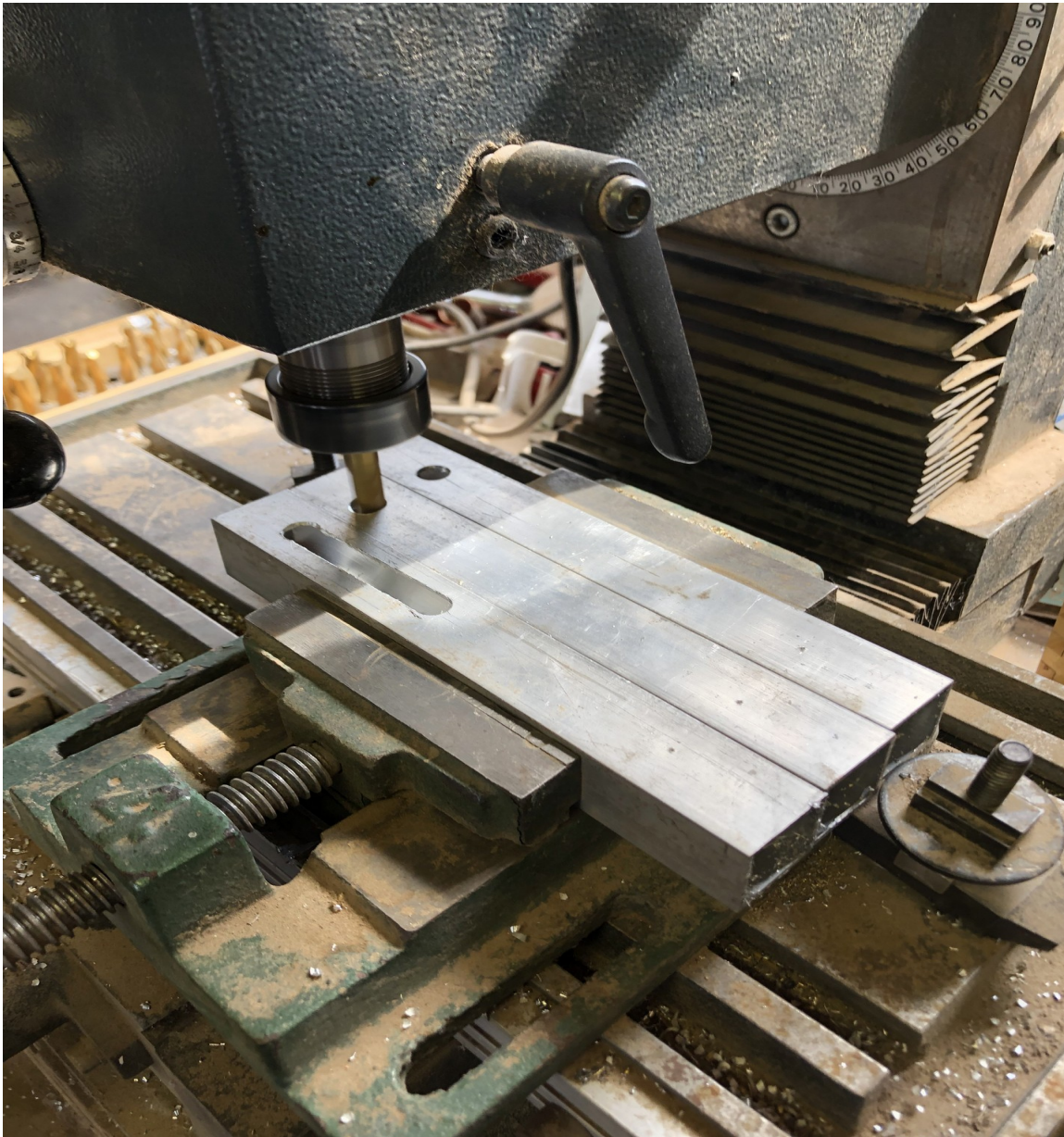
Figure IV-22. Slots being milled into square aluminum tubes that will become adjustable feed horn supports.
