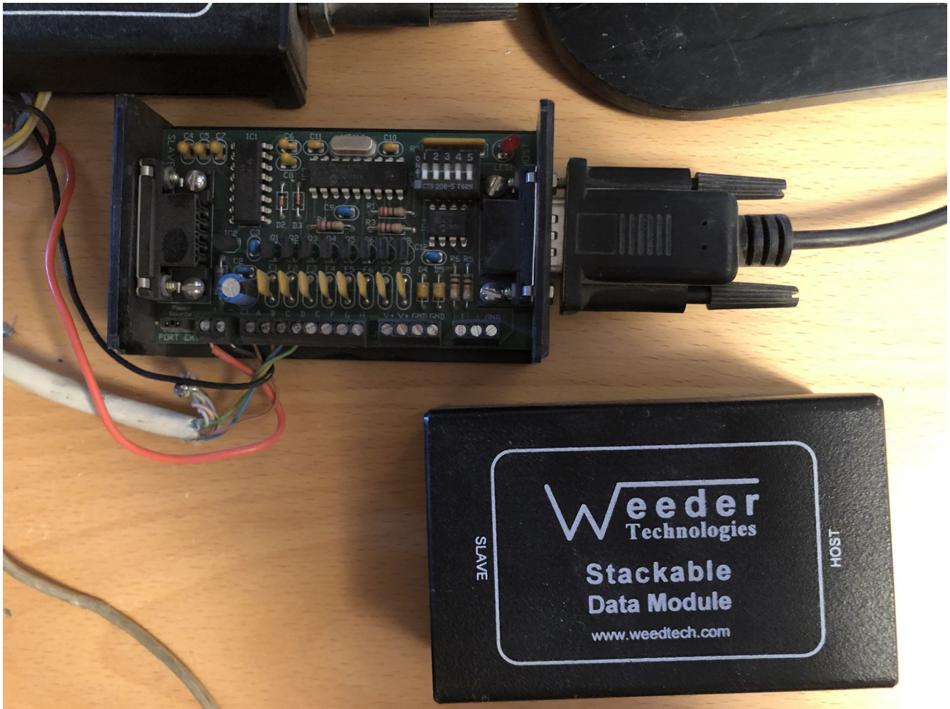
Figure IV-16. The Weeder Technologies WTDOT-M digital output module used to interface the dish motion control panel with a general purpose USB port of the dish tracking computer.
