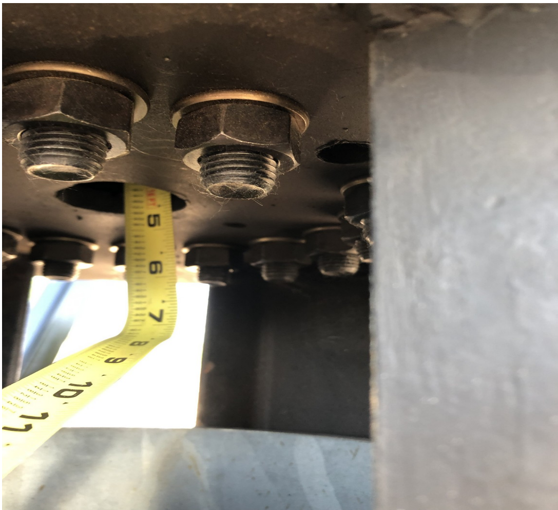
Figure IV-2. Measurement of the distance between the rotating and stationary plates of the AZ slewing bearing.
