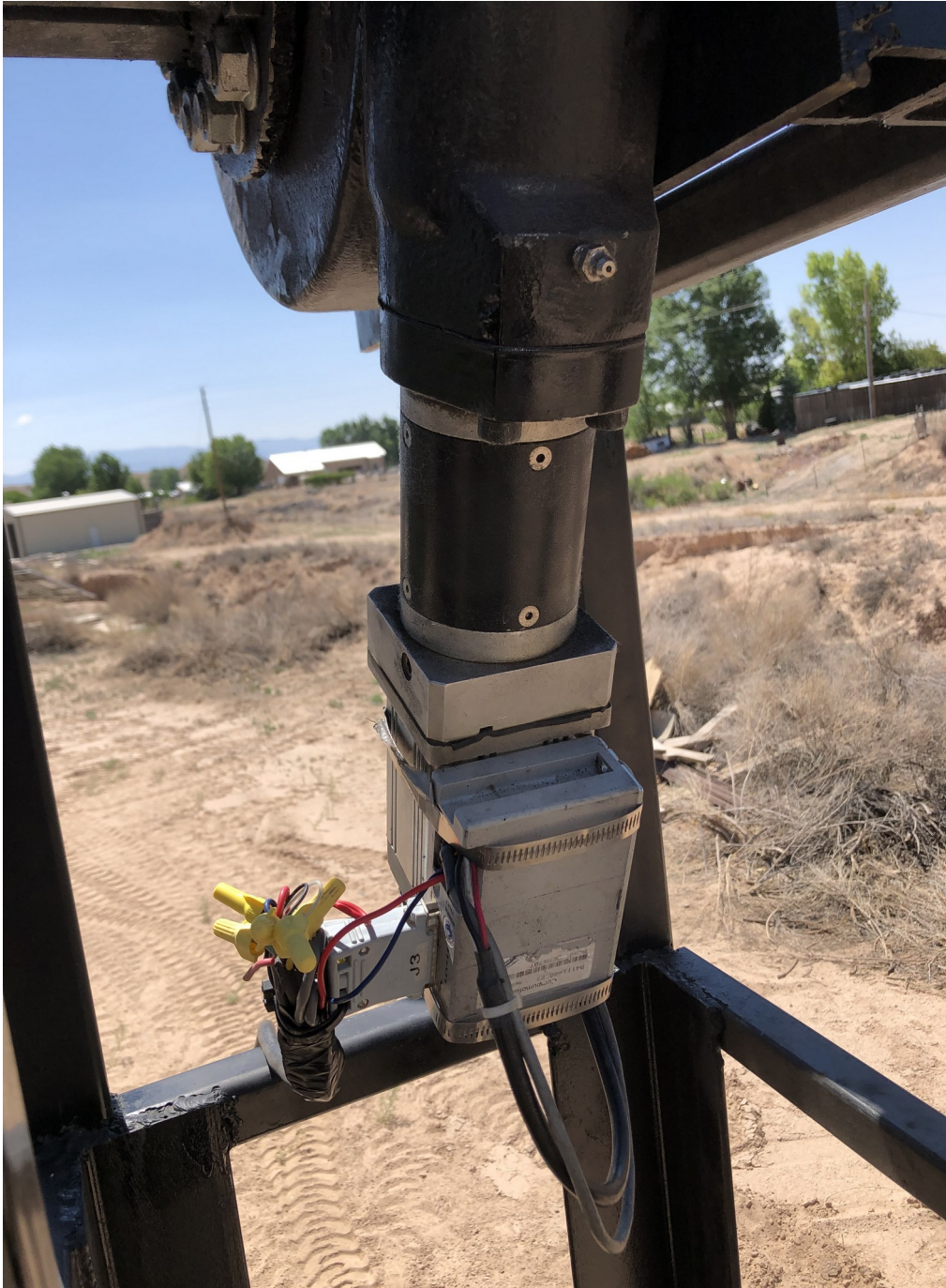
Figure IV-12. The EL servo-motor driver module is strapped onto and below the EL servo motor and temporarily wired to the EL motion control lines from the telescope control room.
