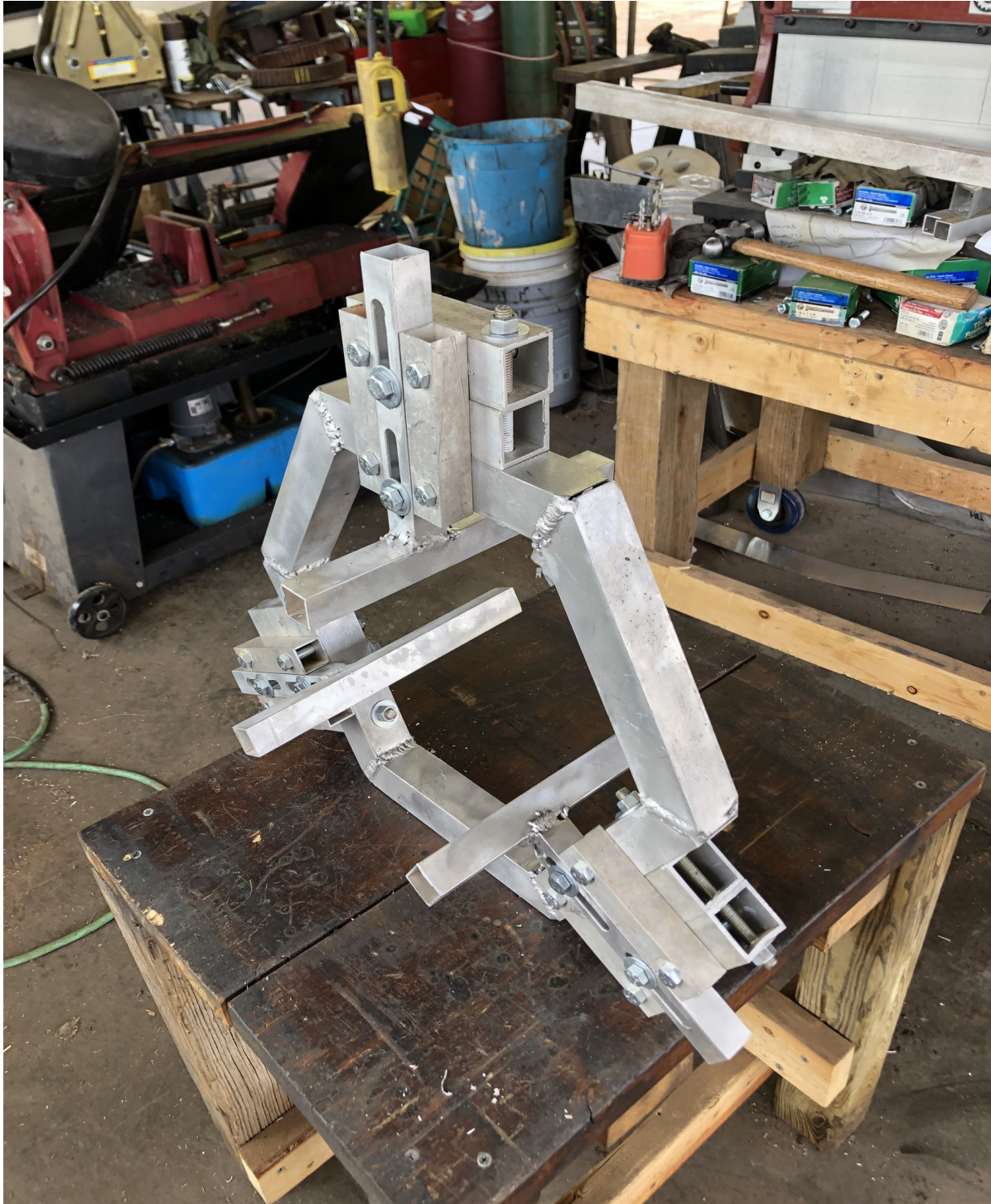
Figure IV-29. All three adjustable feed horn supports are now fabricated and installed on the hexagon ring.
