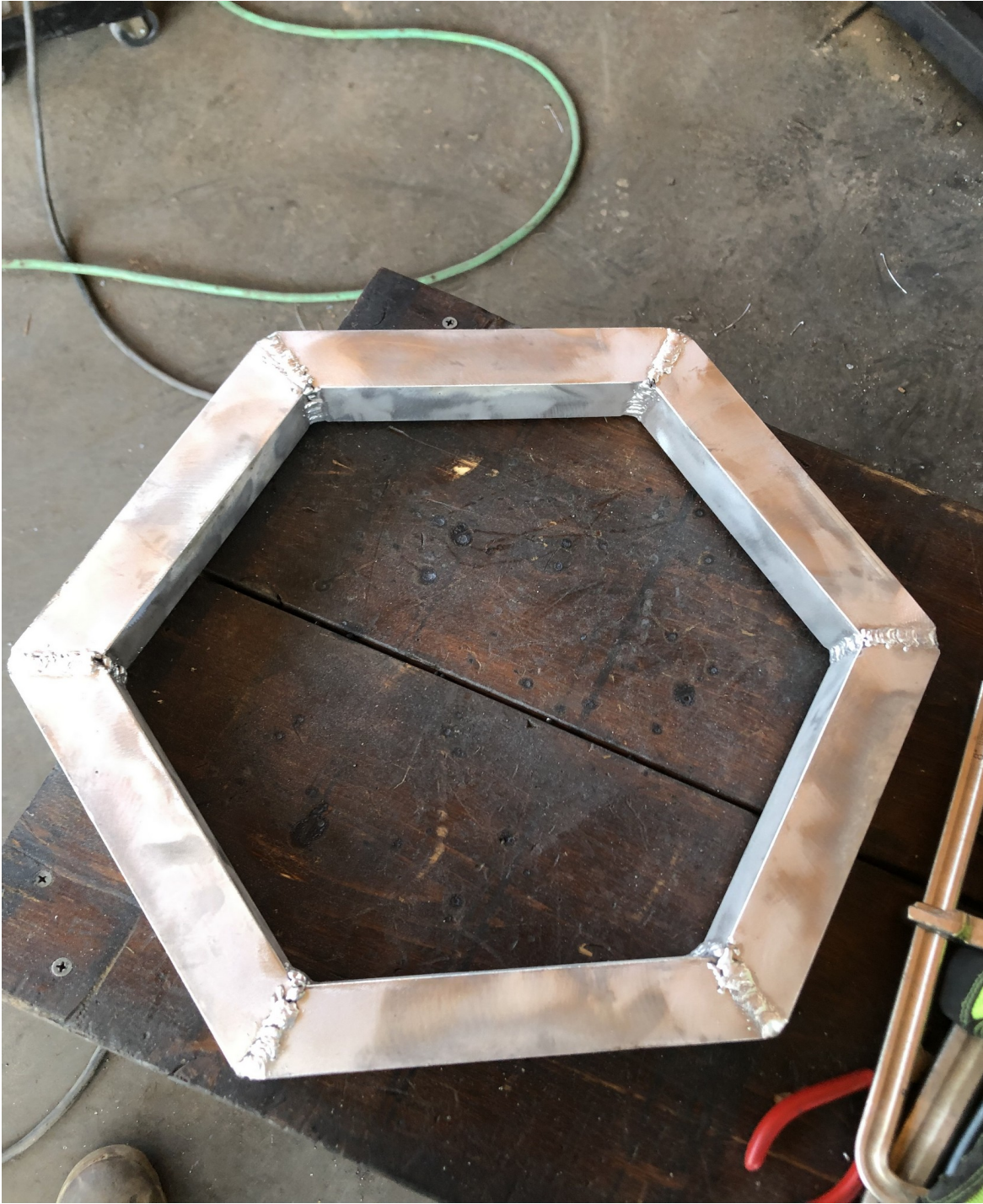
Figure IV-21. The hexagon feed horn mounting ring sides are welded together.
