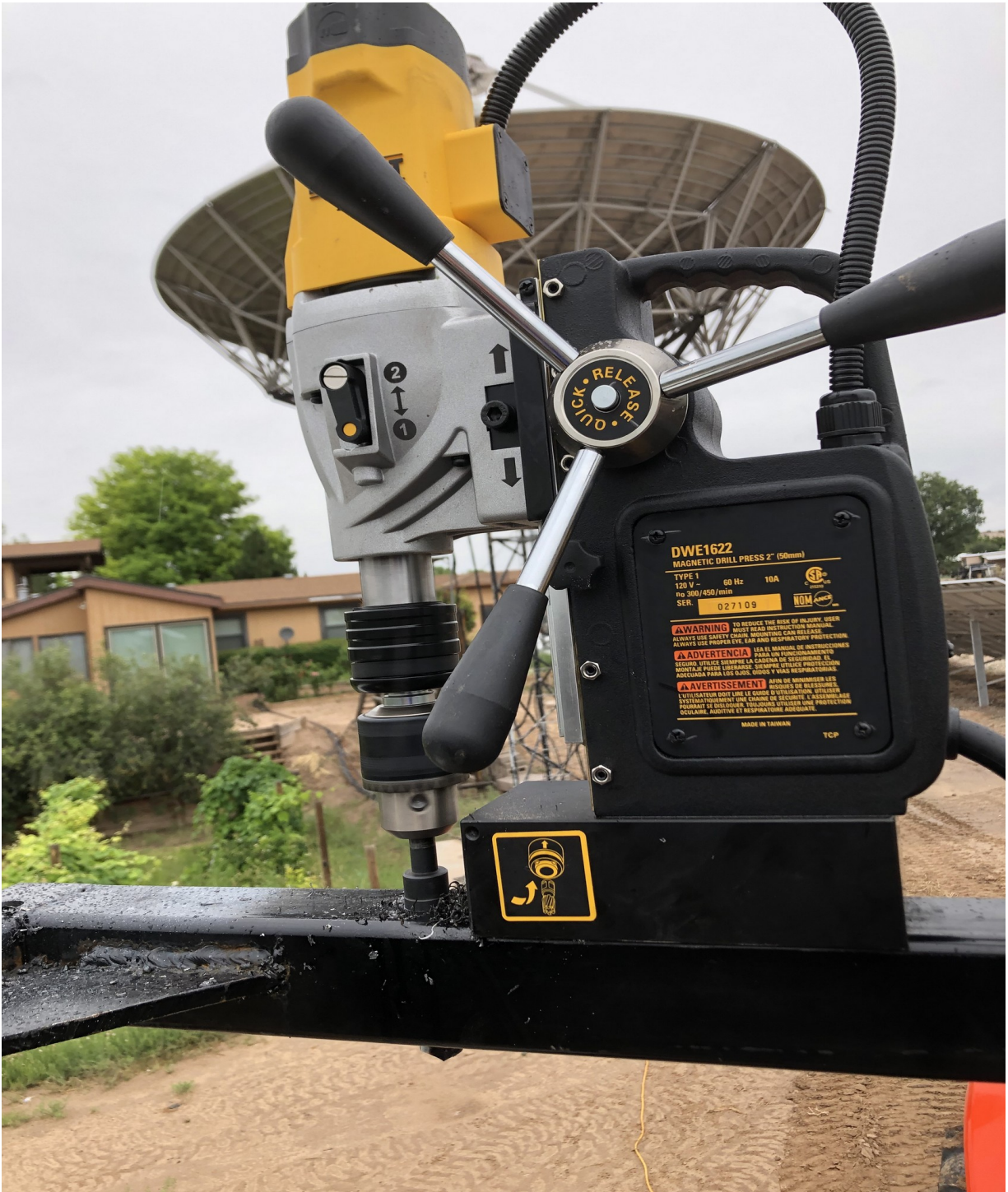
IV-58. A 7/8” diameter through hole has been drilled using a magnetic drill press.
