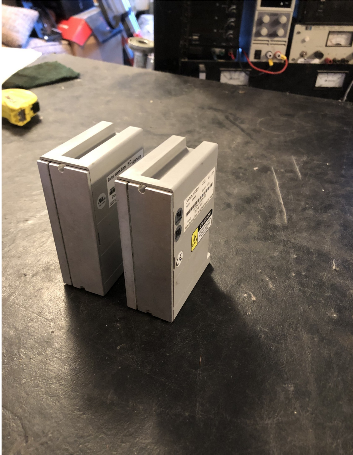
Figure IV-9. Parker OEM670T servo-motor drive modules that are being used to drive the AZ and EL servo motors in this project.
