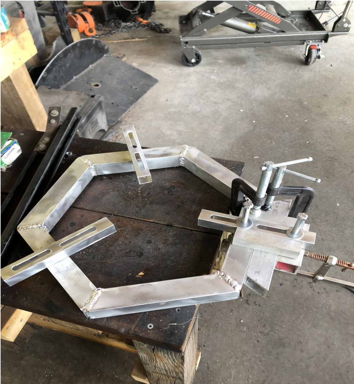
Figure IV-23. Photo showing how the slotted feed horn supports will be attached to the hexagon ring.
