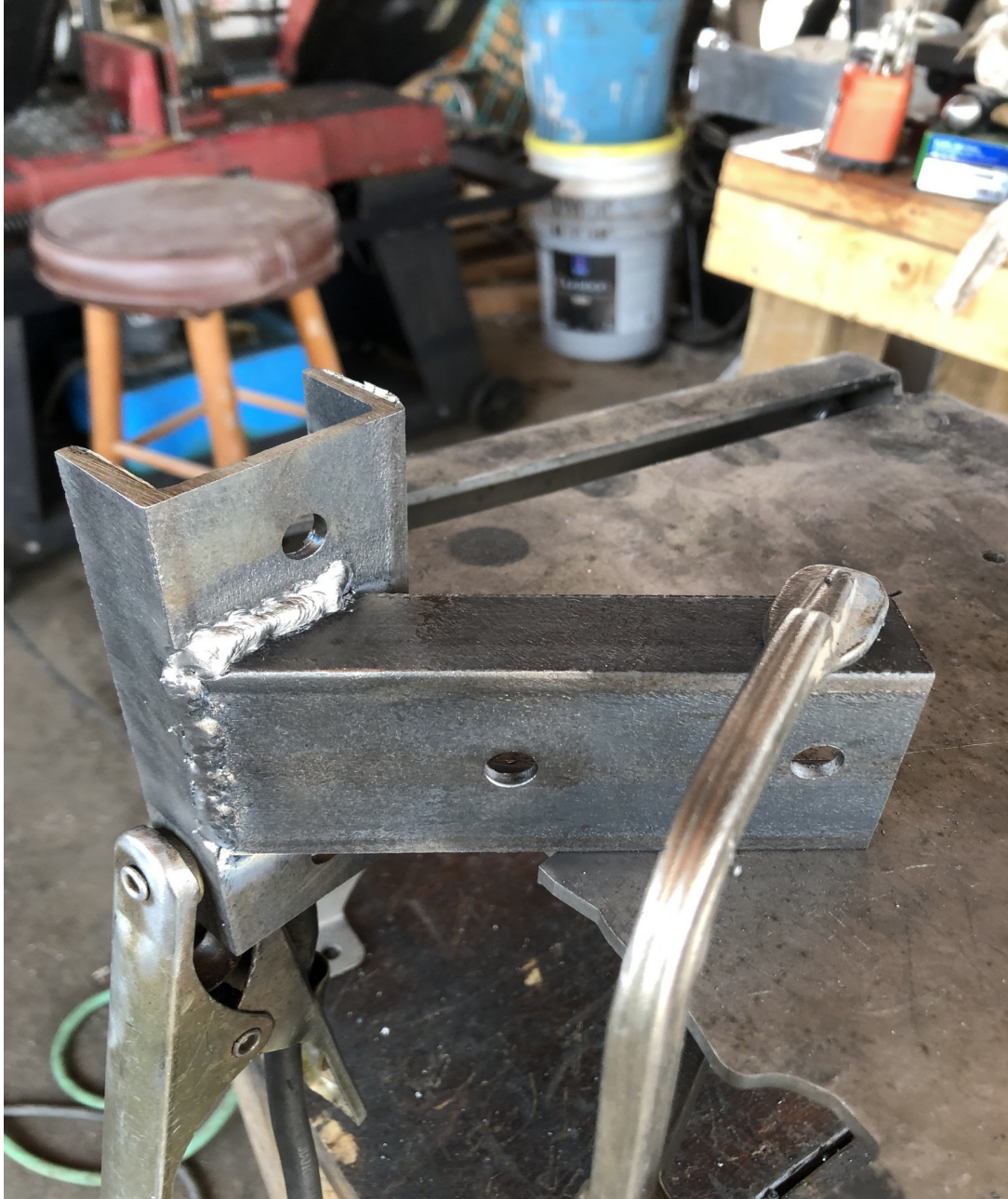
Figure IV-34. An upper end bracket after welding.
