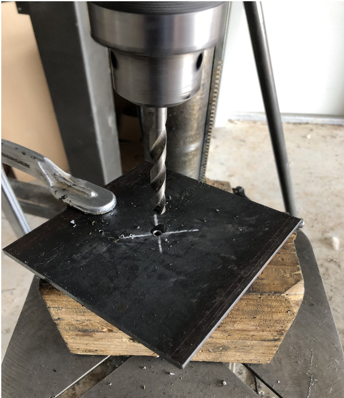
Figure IV-49. Drilling a center bolt hole in one of the rigid template plates.
