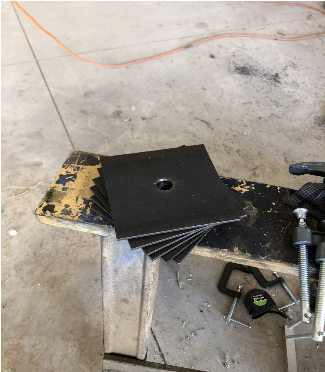
Figure IV-50. Center bolt holes have been drilled in the six rigid template plates.
