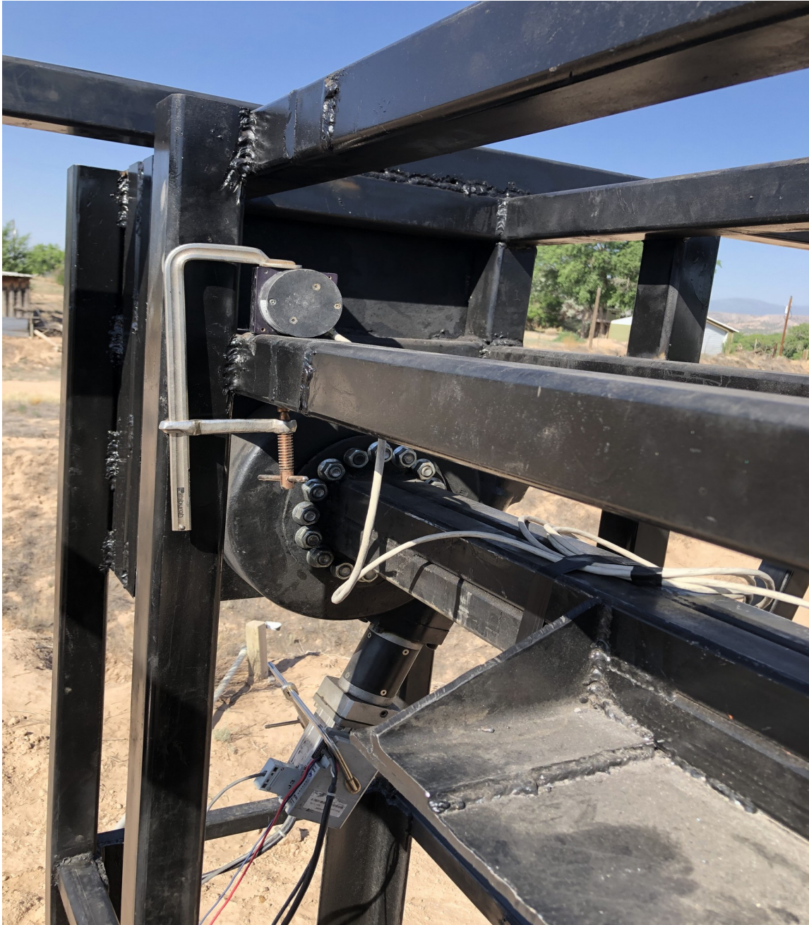
Figure IV-7. EL encoder temporarily clamped onto the EL mount for testing.
