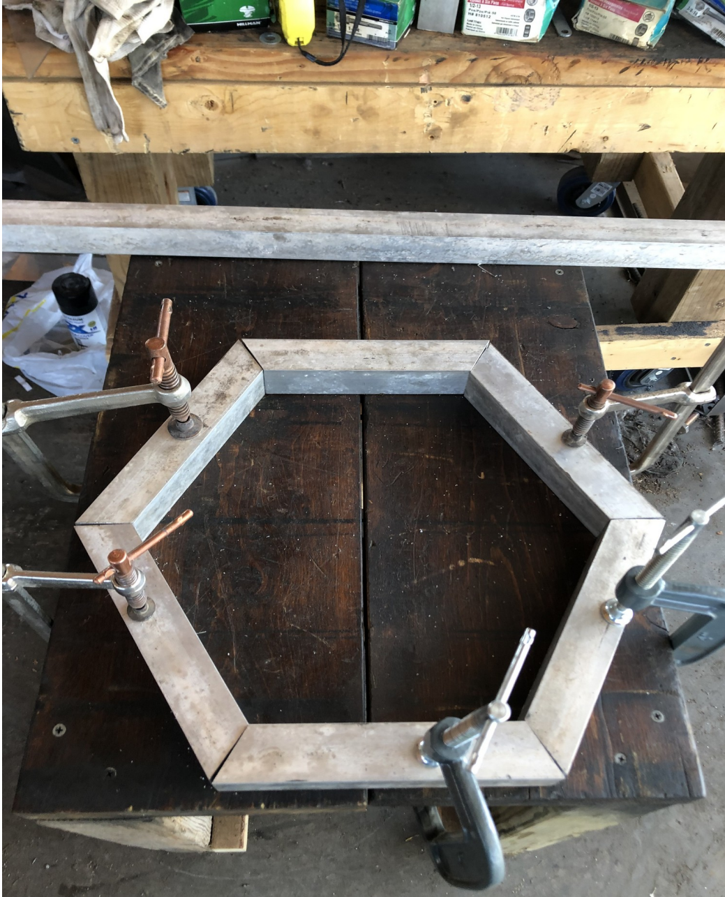
Figure IV-20. Hexagon mounting ring components are clamped into position for welding.
