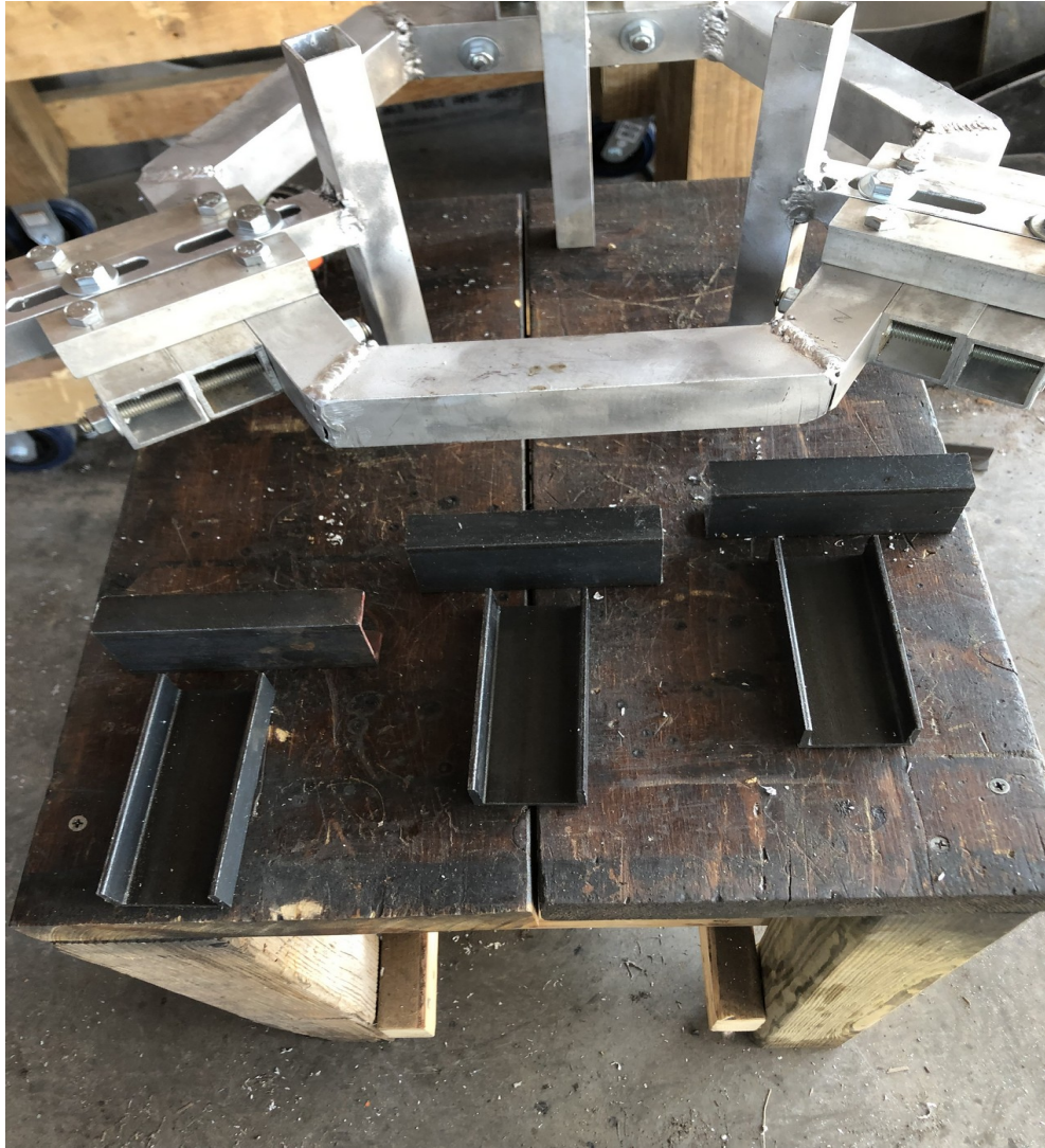
Figure IV-30. Channel iron pieces cut for the upper end bracket fabrication.
