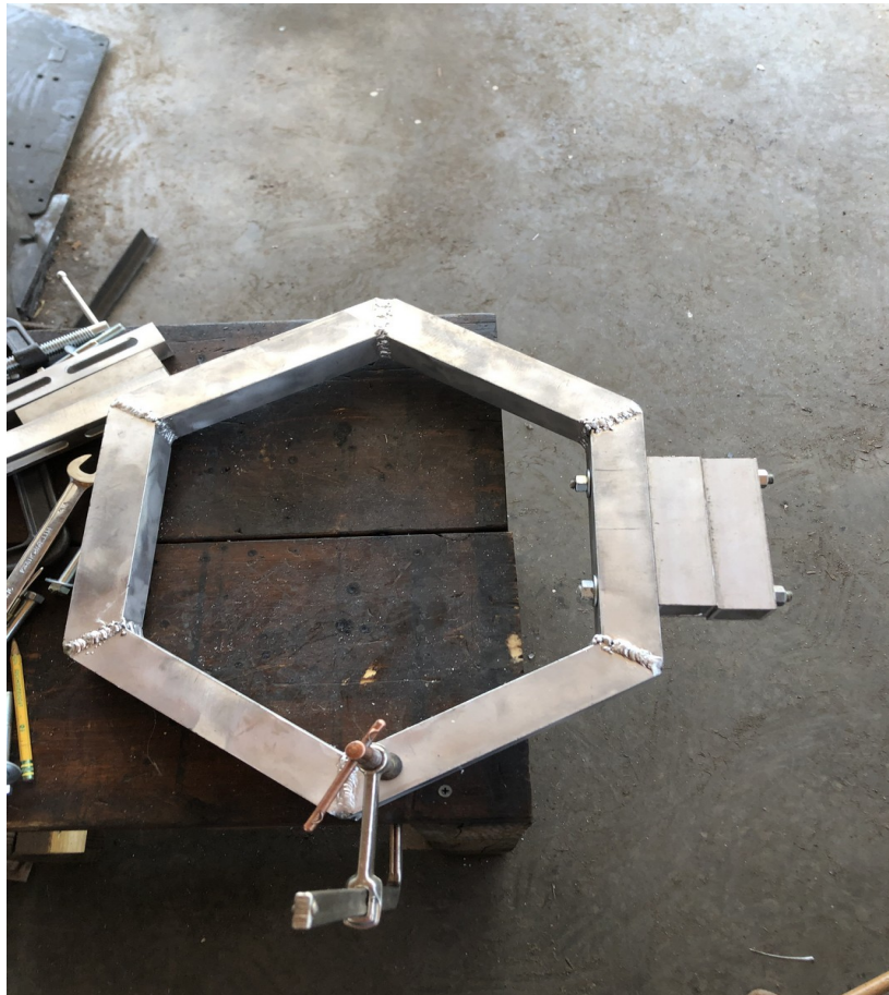
Figure IV-25. Two spacers are bolted to a side of the hexagon mounting ring.
