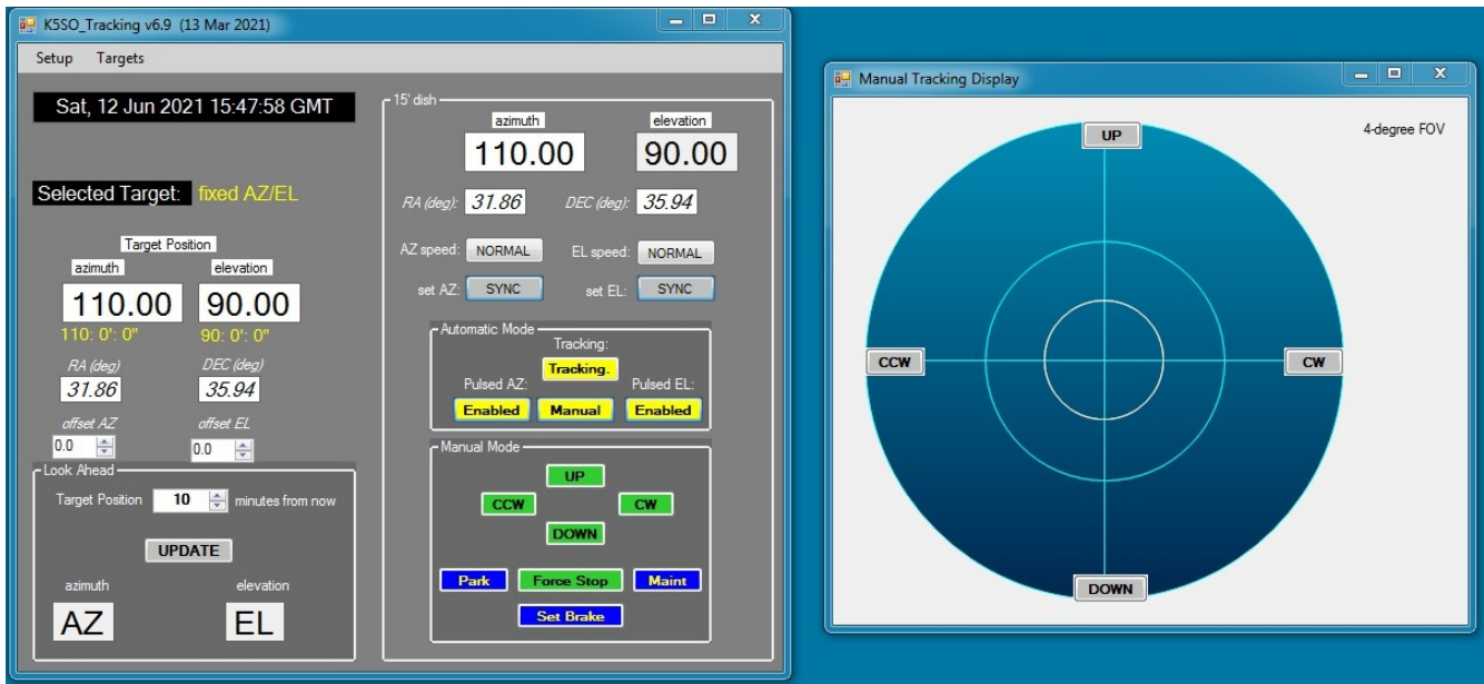
Figure IV-8. Tracking program testing of the AZ/EL encoders in the control room showing that both encoders are functioning properly.
