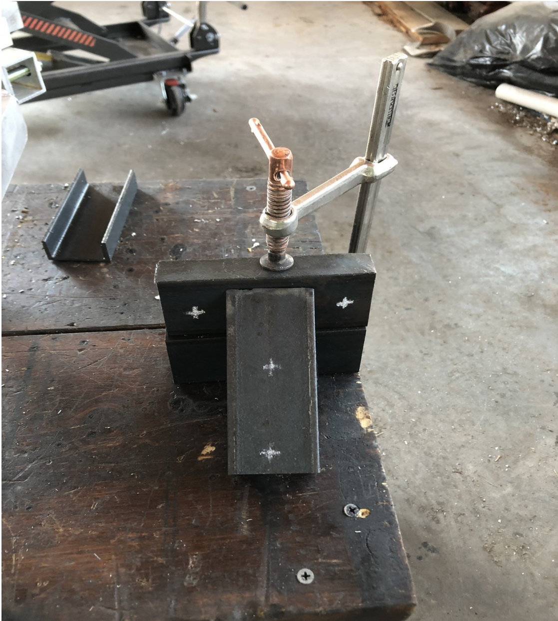
Figure IV-32. Fitting of two elements together for an upper end bracket, with drill hole positions marked for the attachment bolts.
