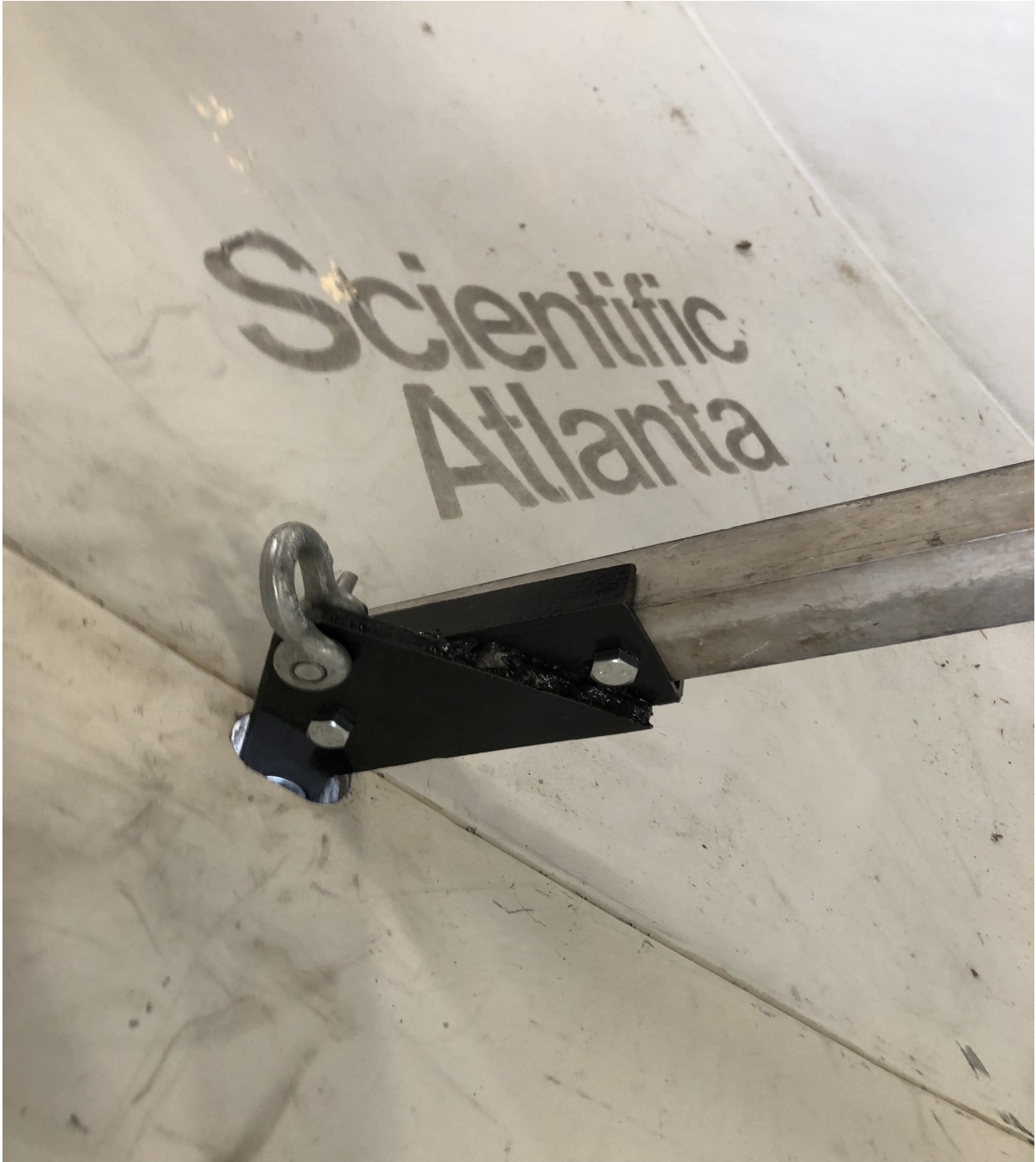
Figure IV-45. A completed lower end feed support arm bracket installed onto a support arm including a utility clevis for later use in lifting the dish into position.
