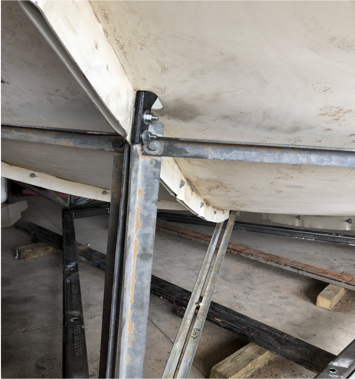
Figure IV-44. A view showing how the lower end support arm bracket bolts onto the steel dish back structure.
