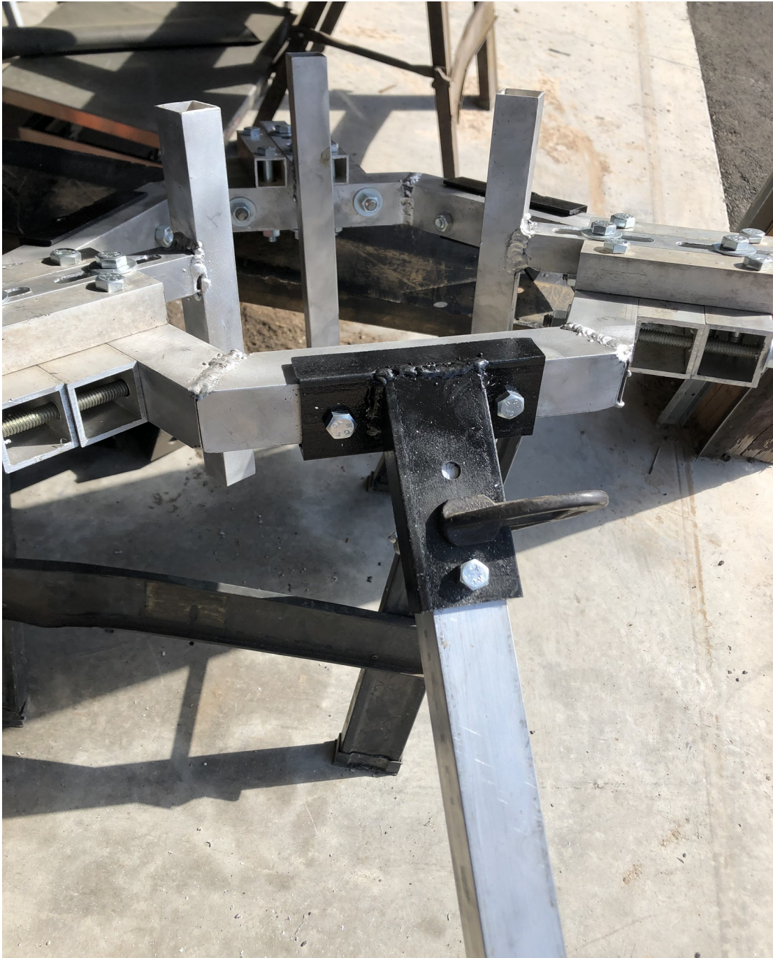
Figure IV-37. Long feed support arm being drilled and bolted onto the hexagon mount.
