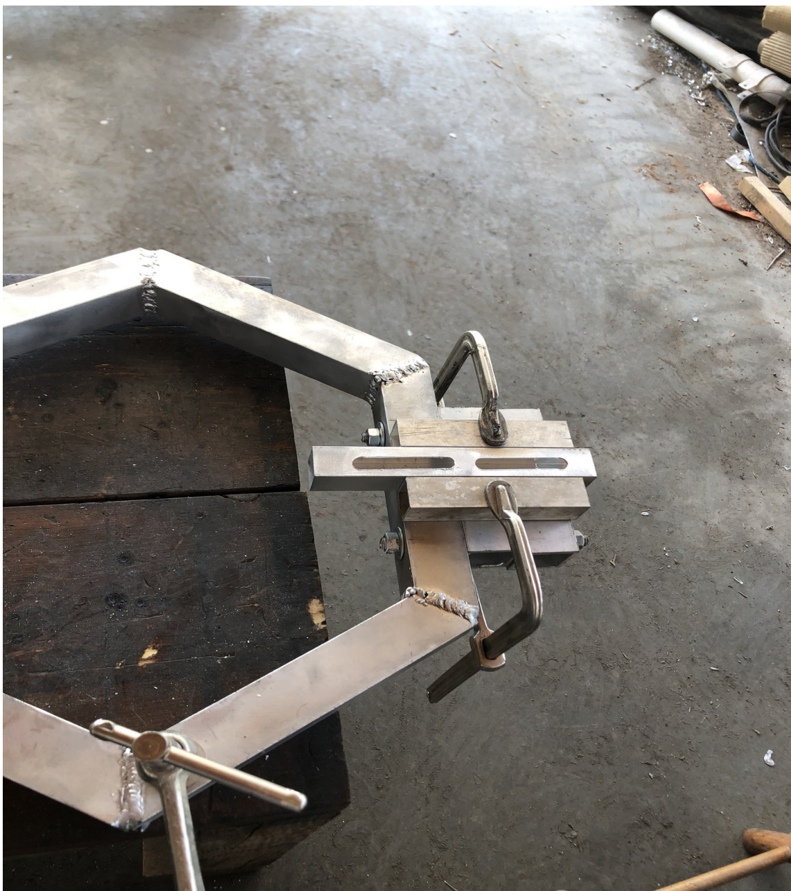
Figure IV-26. The two guides for the slotted support are clamped into position ready to be drilled and bolted onto the spacers and hexagon.
