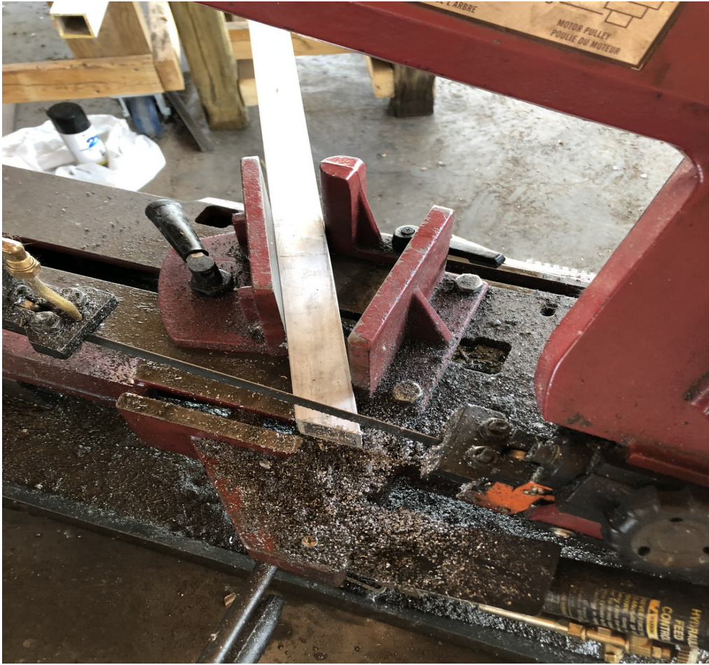
Figure IV-19. Cutting a 30-degree angle for an end of a side of the hexagon mounting ring.
