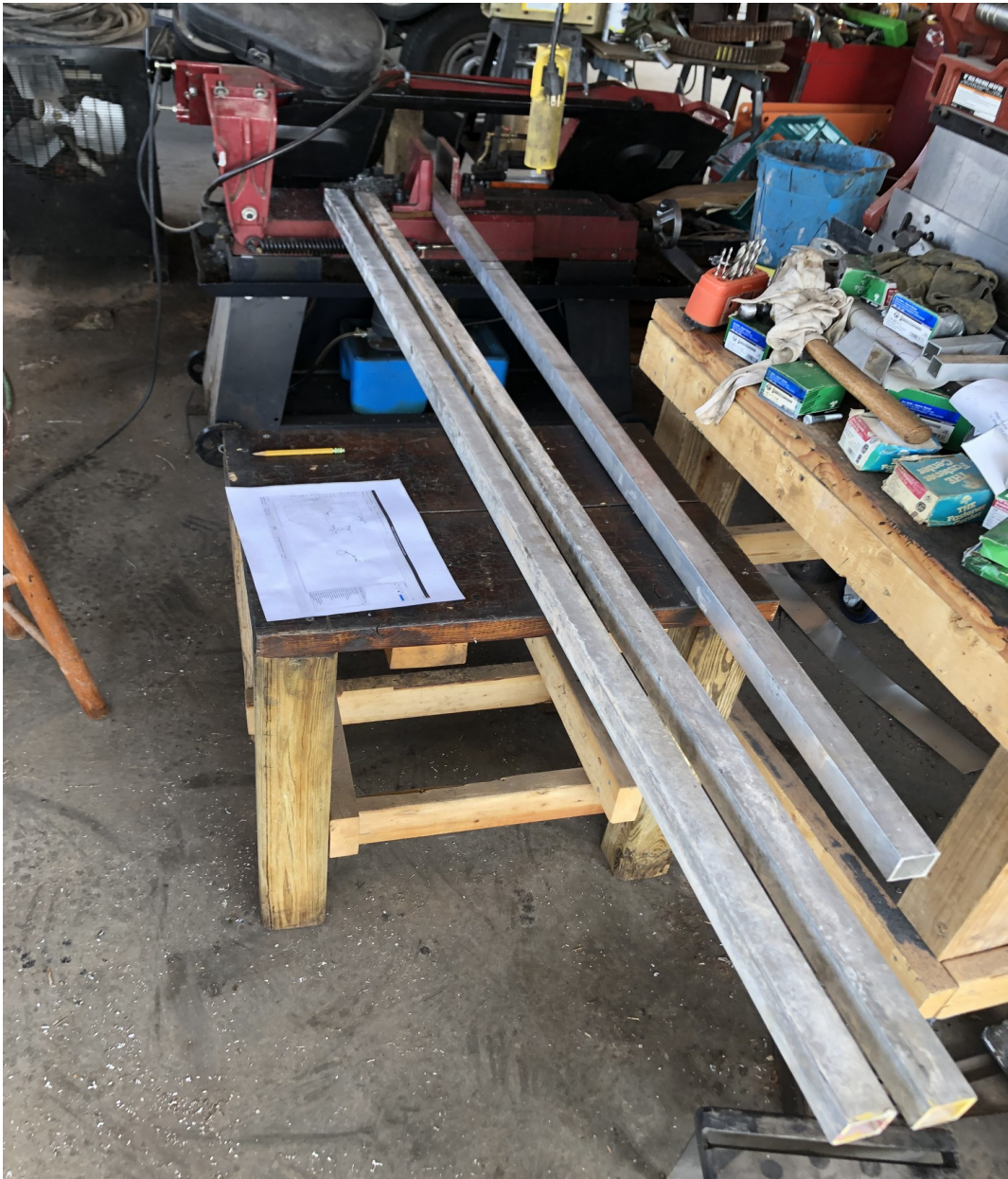
Figure IV-36. The three feed support arms being cut to length.
